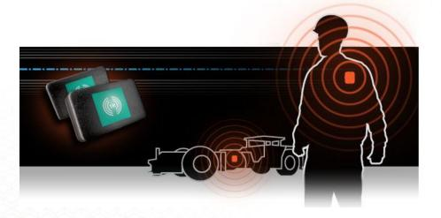
The tag transmits data containing ID, age, activity and temperature for monitoring and reporting purpose. Transmission range is approximately 400 feet per standard reader.
